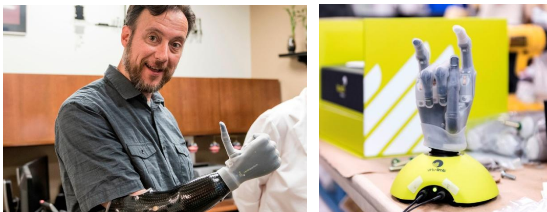
Veteran Daniel Glanz shows off the new prosthetic hand, an iLimb Quantum, which he received at McGuire VA Medical Center. The iLimb Quantum has dozens of modes used to make the prosthetic hand hold a wide variety of different poses.
