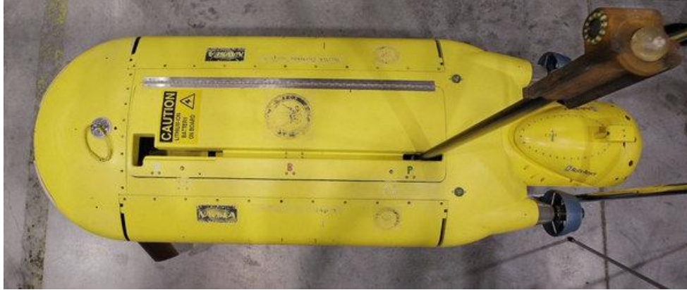
The "Razor," an autonomous underwater vehicle (AUV) sits in a lab at the Naval Undersea War Center in Middletown, RI.
