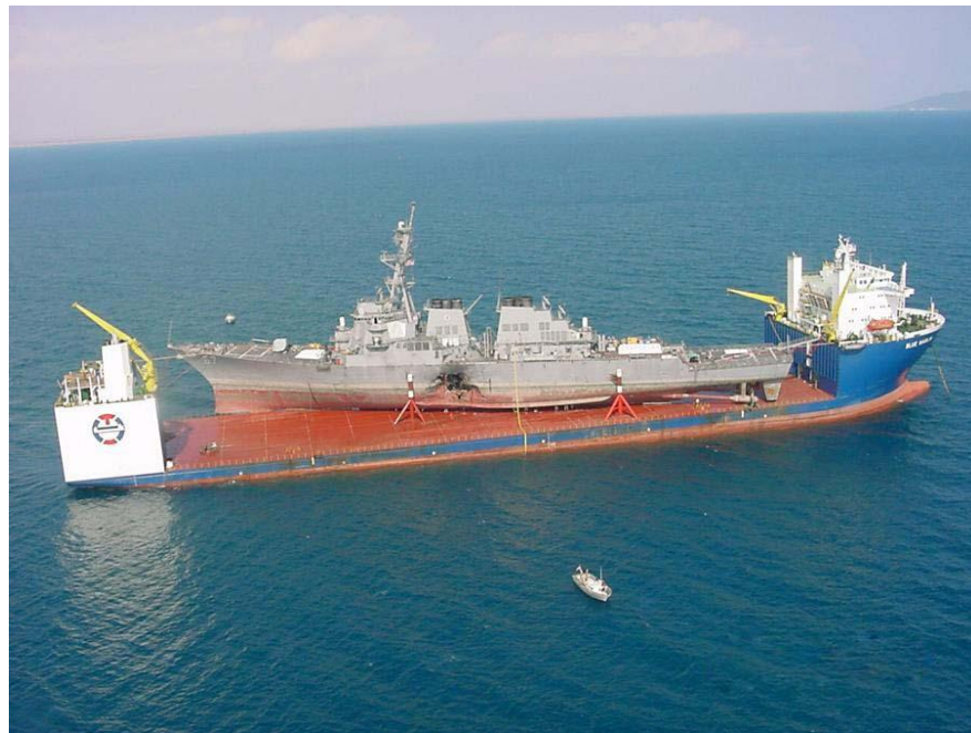
MV Blue Marlin transporting USS Cole from Yemen following the 2000 attack on the ship
